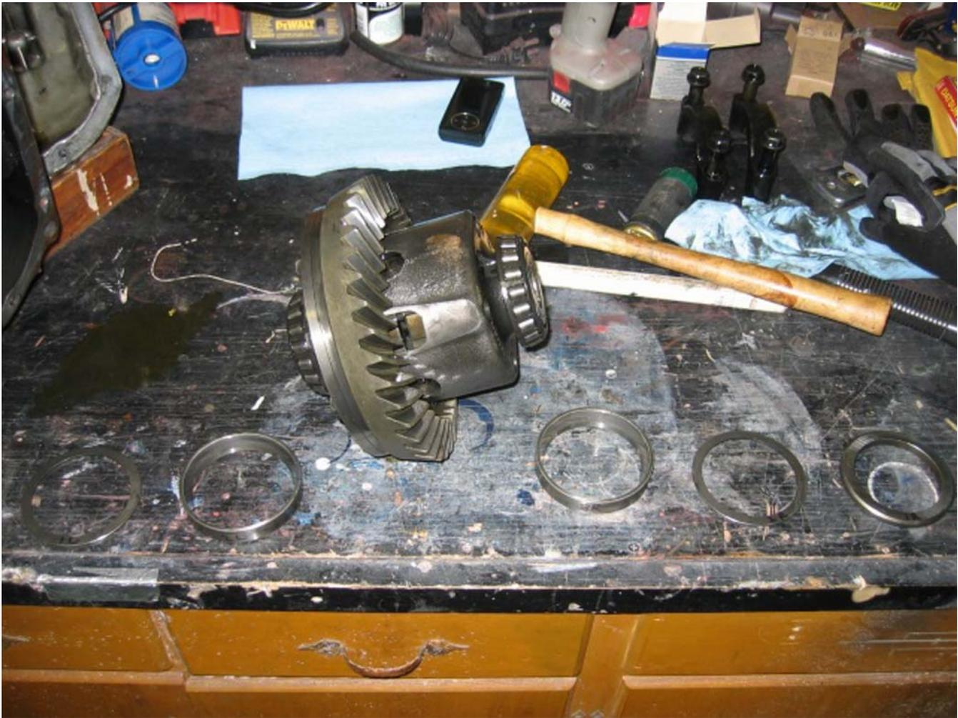
Next remove the ring gear. Once the bolts are removed, it should slide off fairly easy with a few taps from a rubber mallet. I marked the position of mine relative to the LSD housing for safe measures. Once the ring gear is removed you will gain access to the four phillips screws that hold the unit together.
