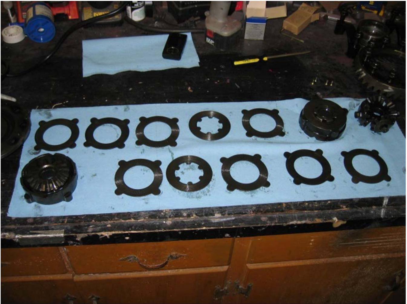
The discs with internal tabs are the clutches. The discs on the ends that look like plates are springs they are dished (kinda hard to see in the picture)
