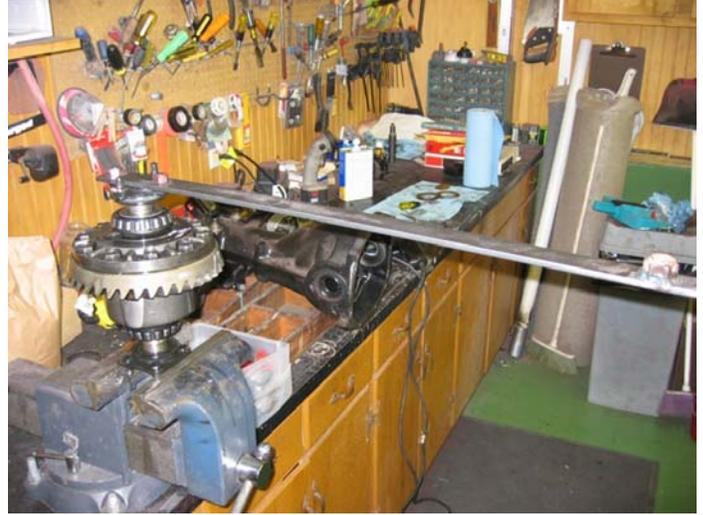
I used a cheap (\$10) beam style torque wrench from autozone to make the measurements. It was placed on the bar at the welded nut you see in the picture. All differentials are going to give slightly different results based on the wear of the clutches and the thickness of the new clutches along with the amount of friction provided by the type of oil you use,
