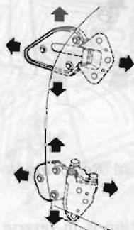
Fig. BF-28 Adjusting Door Alignment
