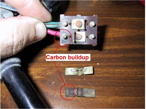
Using the sandpaper thoroughly clean the carbon deposits from both the plates and the contact points that the wires are soldered to. Note that the bump on the plates is in
