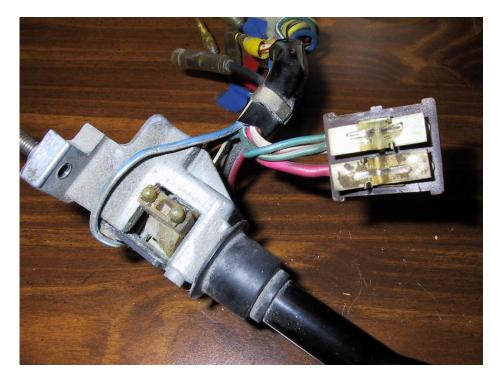
Carefully pop these two plates out. They are the reason your switch is intermittent and need to be cleaned up. Notice the carbon build-up where contact is made
