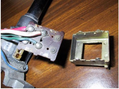
You'll notice two rocker contacts plates that actually close the circuit. Others have mentioned needing to repair/build up the two small spring loaded nubs that actuate the switch. These not only push on the plates to close the circuit but also provide the detents
