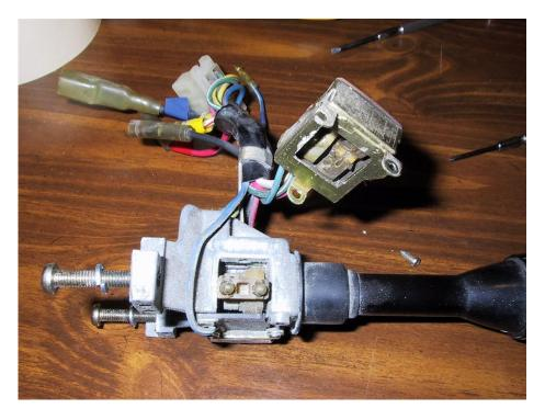
Next, using the flat blade or chisel, carefully pry up the four tabs the hold the circuit board to the box and remove the box.
