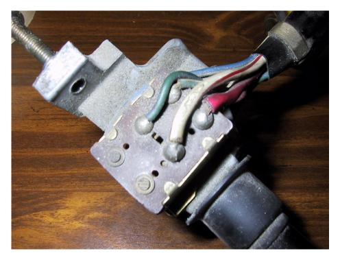
I first took off this entire box by removing the 3 screws that hold it on. This step might not be necessary but it probably makes it easier. Be careful not to lose the small plastic washer that fits in one of the 3 screw holes. Also, note that the shorter of the 3 screws goes on the side where the wires come from.
