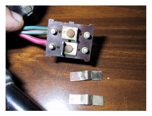
Re-assembly is the opposite of disassembly. Use your ohm meter to verify that the switch is now as good as new.
